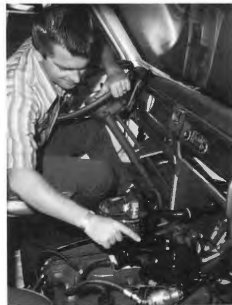
COMPACT UNIT —Jim Michlec points to the pressure regulator which changes the liquified propane to a vapor.
