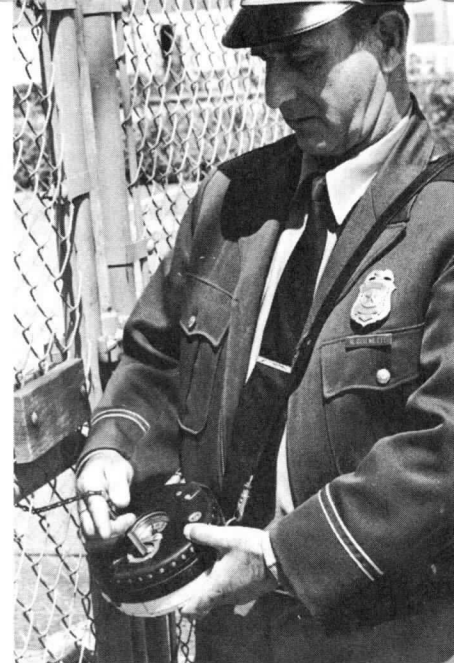
Security and insurance regulations require frequent specified checks of all locations throughout Data Systems. Ronald Guilmette inserts a key in a detex clock imprinting the key number within the time element of the clock to record security check.
